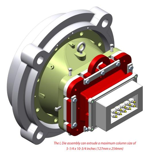
The Steele L Die combines innovation and flexibility in a high-efficiency stiff extrusion die system. It's the first die with a bridge that can be removed from the front for fast changes. The overall length and internal profile varies with mid-base and shaper cap options, making the L Die well suited for a range of raw materials and products.
