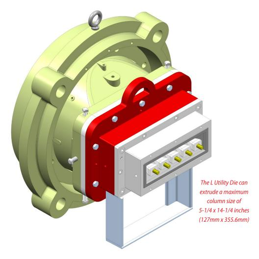
The L Utility Die offers the innovation and flexibility of the L Die, with a design that produces utility brick and extrusion profiles up to 14" (356mm). Front bridge replacement permits fast changes and adjustments during operation. Mid-base and shaper cap options extrude a range of low-moisture raw materials and products. The bridge features a high carbide coating, for a service life four to five times longer than competitive designs.
