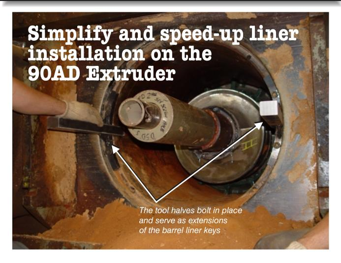
This tool bolts onto the front flange of the hydraulic die changer main frame. Liner adapters or adapter/circular liner assemblies can then be centered and aligned for installation in a more convenient location.
