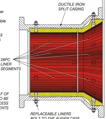
**BOLT TO THE AUGER CASE** (hardcaking problems can be treated by adding water through the liner bolts)
