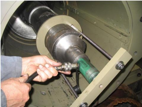
7. Blocks must be used between the port-a-power and the pulling cross bar as the gap increases.
