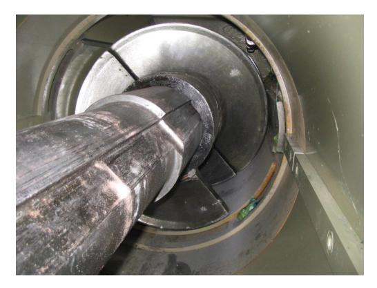
2. Insert one of the short hooks into the auger pulling pocket as shown. This is simplified if the augershaft keyway can turn to the 12 o'clock position. Do this by sliding the rod with the hook turned flat and then rotating the rod counterclockwise, engaging the hook in the auger pulling pocket. This is illustrated in the following pictures for the number 5 auger.
