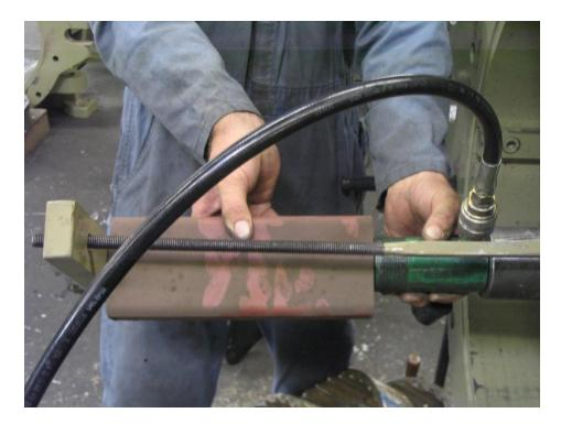
8. Use the port-a-power until the auger can slide freely to the end of the auger shaft by hand. Use extreme care when removing augers from the shaft.
