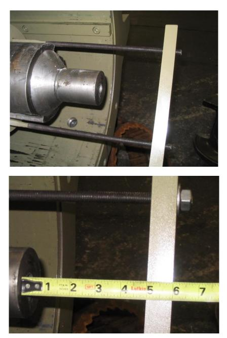
6. Position a hydraulic port-a-power (not supplied by Steele) between the end of the augershaft and the pulling cross-bar. The estimated minimum gap between the pulling cross bar and the end of the augershaft is 5 inches.
