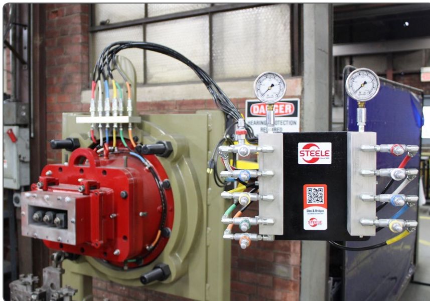
A remote die oil manifold articulating arm improved die lubrication and operator safety
