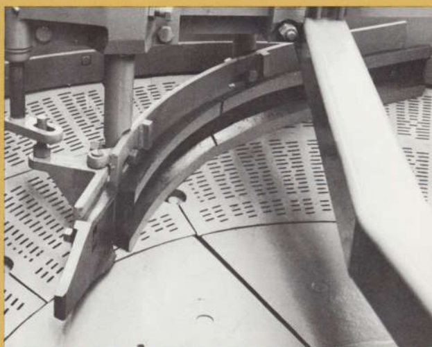
Fig. 12 Adjustable Blade on Spiral Scraper
