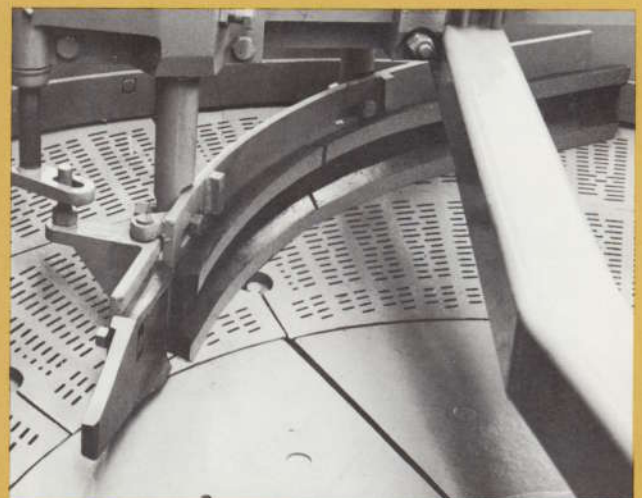
Fig. 12 Adjustable Blade on Spiral Scraper
