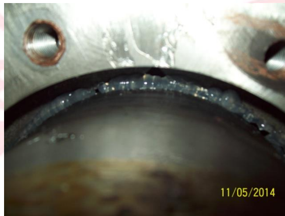
FIG 4: Sealing core with packing installed
