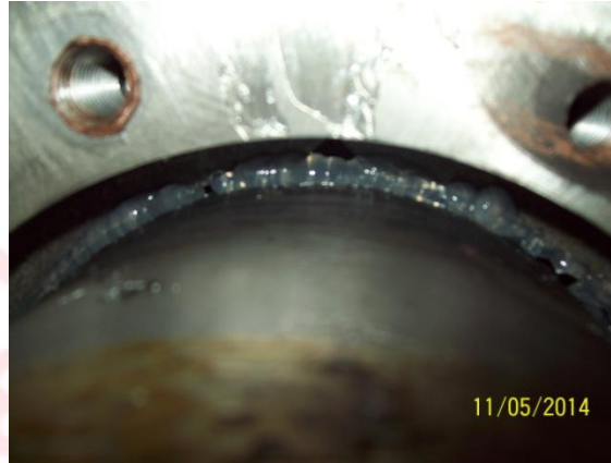
FIG 3: The second possible leak pathway is between the inside of the sealing core and the shaft. This normally is sealed with the packing. Again, silicone can be used prior to installing the packing to increase the certainty that vacuum is sealed. A silicone bead has been applied between the shaft and sealing core inside diameter at the bottom of the groove where the packing will seat. Alternatively, silicone can be applied to this region before the sealing core halves are installed on the shaft.
