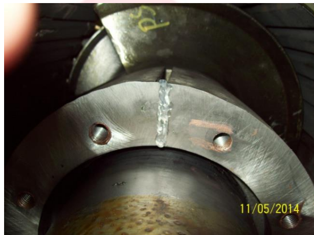
FIG 2: There are two possible avenues here for a vacuum leak. The first leak pathway is the two splits. These normally fill with material (clay, shale, etc.). In these photographs silicone has been applied into the casting splits. This silicone and the raw material (clay, shale, etc.) that will fill in behind it will seal for vacuum here.
