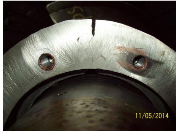
FIG 1: The exit end of the sealing core, as viewed from the pug sealer vacuum chamber. The “split” shown is oriented at the top position. The other split (not shown) is at the bottom position.
