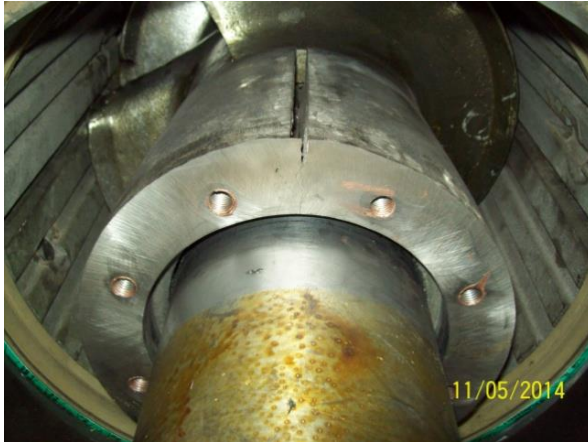
FIG 1: The exit end of the sealing core, as viewed from the pug sealer vacuum chamber. The “split” shown is oriented at the top position. The other split (not shown) is at the bottom position.
