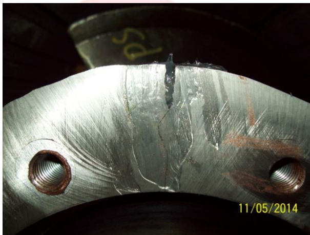
FIG 2: There are two possible avenues here for a vacuum leak. The first leak pathway is the two splits. These normally fill with material (clay, shale, etc.). In these photographs silicone has been applied into the casting splits. This silicone and the raw material (clay, shale, etc.) that will fill in behind it will seal for vacuum here.
