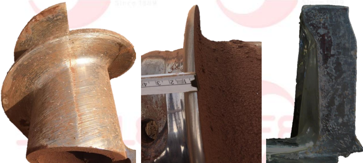
FIG 1: Photos of auger wear
