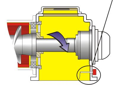
The sensor is optional on new pug sealers and can be retrofitted to existing systems.
