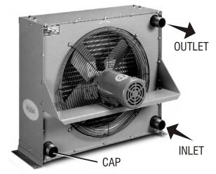
This oil cooler is designed to maintain a service oil temperature below 145° F in the most severe ambient conditions for the Steele 30-HP Vacuum System. When properly installed and maintained, this oil cooler will improve the performance of the vacuum system, minimize the generation of sludge in the oil, and extend the life of the pump seals.
