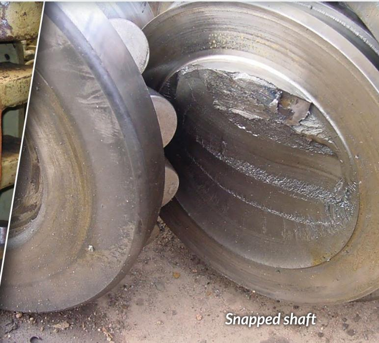
*Better barrel lubrication helps prevent component failure.*
