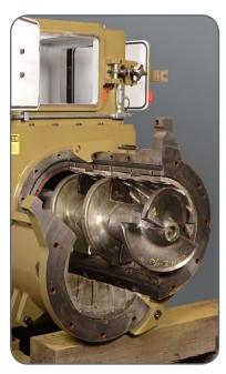
The Steele 45 Extruder offers convenient access to auger spirals and liners.
