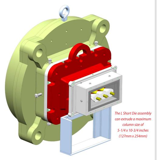
The L Short Die offers the same features of the L Die, using a minimum-length die assembly for plastic materials. The short die length allows fine particles in plastic materials to form more easily, improving compaction and reducing required amperages for energy savings. Front bridge replacement permits fast changes and adjustments during operation.
